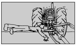
Keep all guards in place when the machine is in operation
