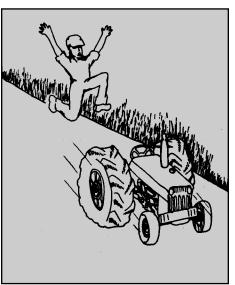
When tractor is stopped, set brakes securely.
