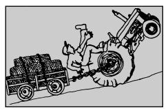
Hitch only to drawbar and hitch points recommended by manufacturer
