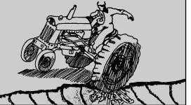
Where possible, avoid operating the tractor near ditches, embankments, or holes.
