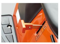
**Four Wheel Drive** Engaged by a single lever, 4WD is standard on the CS Series tractors.
