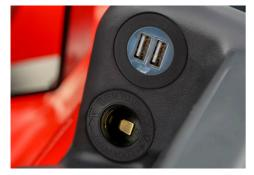
**12V/USB Port** The standard 12 volt power outlet with added USB port is available for accessories.
