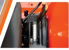
**3-Point Control Lever** The ergonomic 3-point control lever has smooth motion for reduced effort and improved control.
